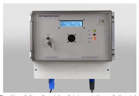
The unit is supplied in a wall mounted case featuring a protective cover for the control panel. It has dedicated connectors for Mains INPUT and Clock OUTPUT, as well as a connection for a single bell hammer and the GPS Antennae which is supplied with the unit. The unit and clocks are supplied to operate from a 220-240v 50Hz supply unless stated otherwise.
